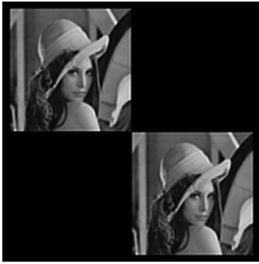
Fig. 5. Double Lena target image ( 512 \times 512 ) with a b = 0.35 low-pass Butterworth filter applied.
